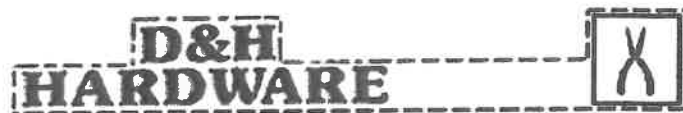
Figure VIII.3-1: Example of how a sign area is determined by drawing a polygon (indicated by the dashed line) around all type and markings associated with the sign.
