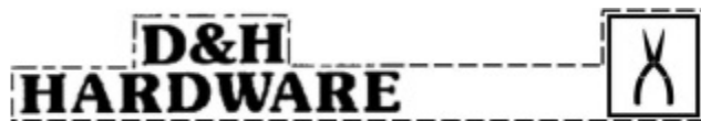
Figure VIII.3-1: Example of how a sign area is determined by drawing a polygon (indicated by the dashed line) around all type and markings associated with the sign.
